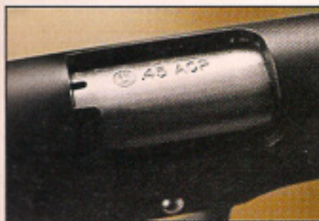
The hood of the barrel has the Para marking and caliber designation. A notch is cut in the hood to allow a peek to check chamber loaded status.
