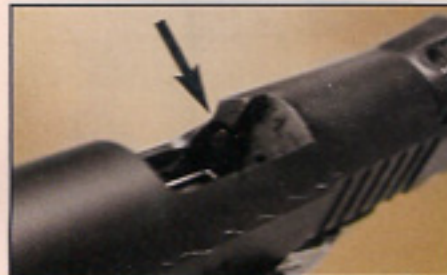
The PXT "Power Extractor" has a comparatively huge claw with which to feed/extract a cartridge case.
