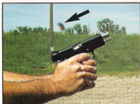
Note the ejected case is barely in the air while the next round is feeding up.
