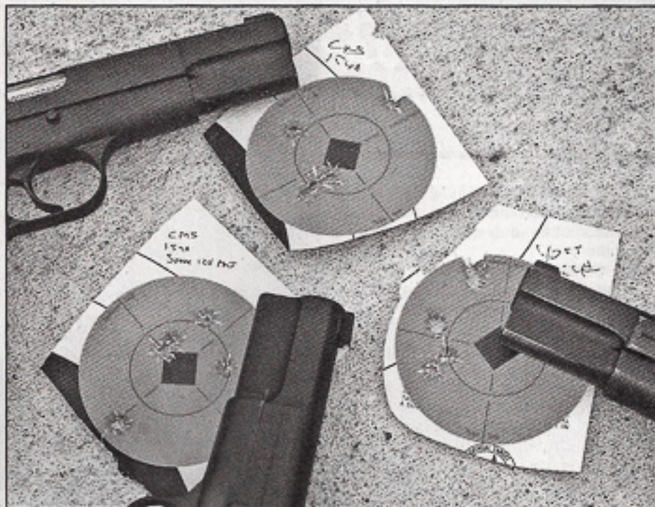
All three shops retained the factory barrel. Groups from 15 yards were well within acceptable accuracy with the major limitation being the author.
