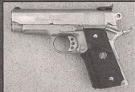
Officer's Model before being customized by Cylinder & Slide. Note stock hammer, MGW (Maryland Gun Works) fixed rear sight, stock front sight, and "shallow" aftermarket beavertail grip safety.
