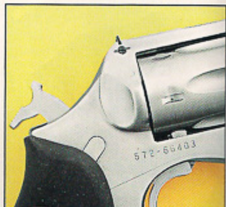
As with other Ruger revolvers, there's no firing pin on the SP101 hammer.
