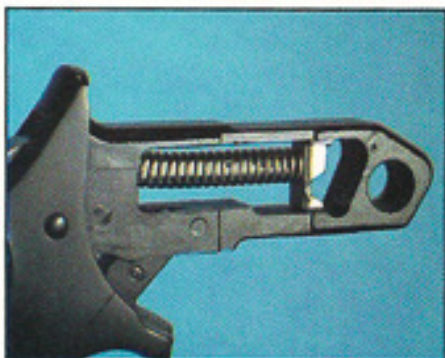
Another feature that adds to the reliability of these guns is the unbreakable coil mainspring (above). Grips are easily removable to begin the field stripping process (top), only a screwdriver is needed for the grip screw.
